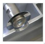
Carbide saw blade for long life and precise sawing.
