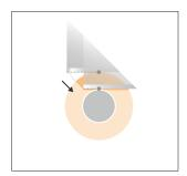
Depending on the processing diameter, the blades have a different contact point on the blade edge. By using the entire blade edge, the life of the blades is increased.
