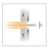
The centering jaws and the blades are programmable for each layer, independently of each other. The blades cut linearly and perpendicularly to the cable axis and are arranged adjacent to the centering jaws.
