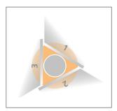
Due to the large contact surface, the 3 knives provide an advantage over a two-knife stripping head when stripping strongly adhering insulations.
