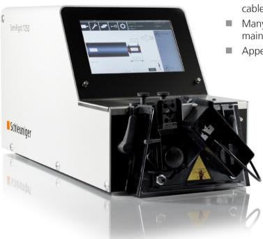
The SemiRigid 1050 is a highly specialized machine for stripping aluminum or copper jacketed semirigid coaxial cables. It features a user-friendly, high resolution color touchscreen interface and intuitive programming. The SemiRigid 1050 offers the precision and flexibility needed to process semi-rigid coaxial cable at the highest possible quality!
