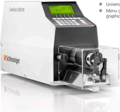
The CoaxStrip 5300 RX quickly and accurately strips wires and cables that would be virtually impossible to strip by hand. The CoaxStrip 5300 RX strips extremely thin micro-coaxial cables down to inner diameters of only 0.07 mm (42 AWG) at short cycle times. Its high-speed rotary stripping head guarantees maximum precision and prevents maintenance-related machine downtime.
