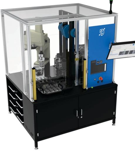
RoSI is designed to insert blind seals and/or hard pins into connectors in a fast and fully automatic way.
