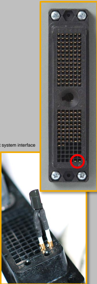
Example: installed data memory in a 156-way ITT Cannon DL1 connector at the adapter cable
