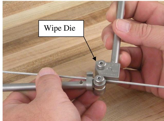
Figure 2: While holding up the back stop with your left hand, close the wipe die with your right hand until it sits tangent to the coax.
