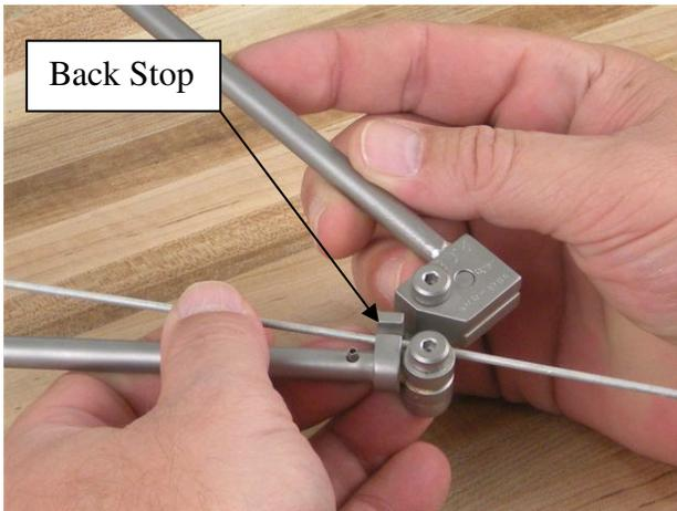
Figure 1: Install coax in bend die groove and then rotate up the back stop as shown with your left ring finger or middle finger as shown.
