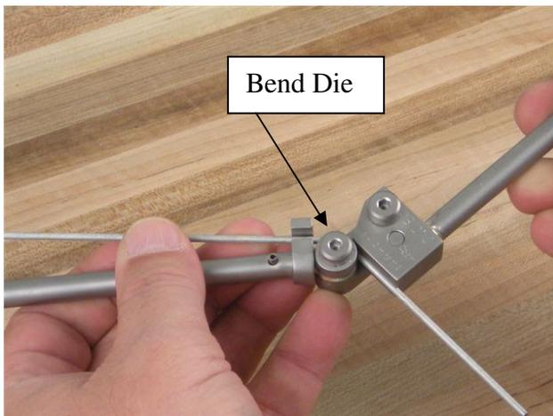
Figure 3: Rotate the wipe die handle CW about the bend die until the desired bend angle is achieved.
