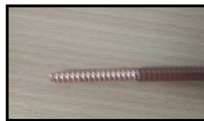
Coroplast cable cleanly stripped using the Mercury-5 laser stripper
