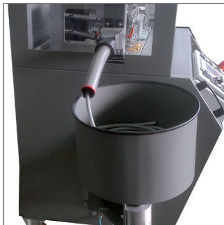
Fig. 3 Coiler pin with adjustable drive motor
