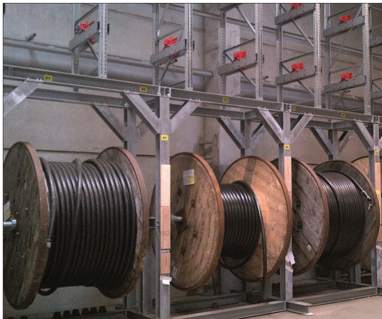
Example: Heavy-load drum bearing and unwinding system combined with LAGROL
