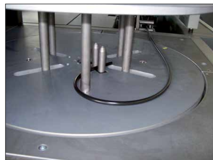
Fig. 4: Cable fixing clamp for coiler head
