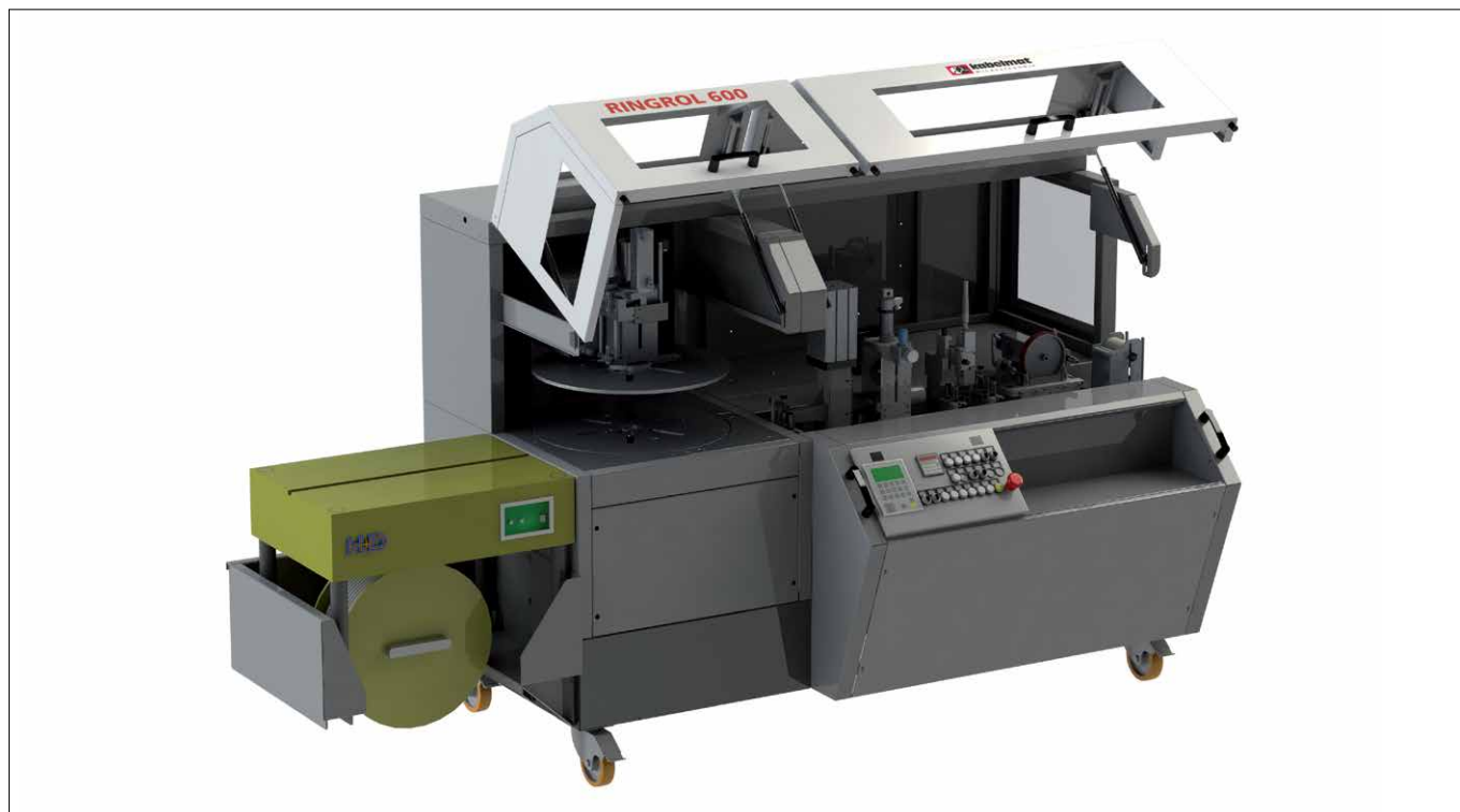
Fig. 1: RINGROL 600 with opened protective cover and biniding unit
