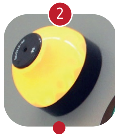
Built-in current leakage detection system for poke-through detection with visual and sound alarms
