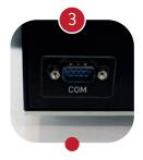
External connection for communication with ultrasonic welding machines, barcode reader or PC programming using Excel™ files
