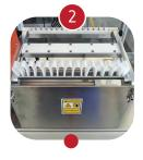
Each workstation can perform, in average, 10 assemblies simultaneously
