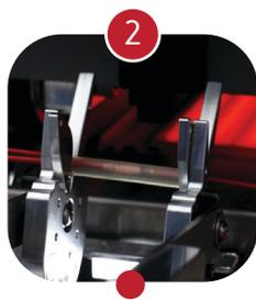
Automatic validation and centering of heat shrink tubes
